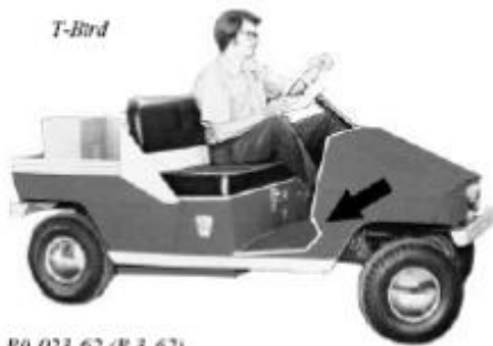
RD-023-62 (R 3-62) GT-023-60 (GT 3-60) Golf car GT-023-61 (GT 3-61) Golf car NOTE: Easily identified by notch in cowling (see arrow). The 370 series does not have this notch.
